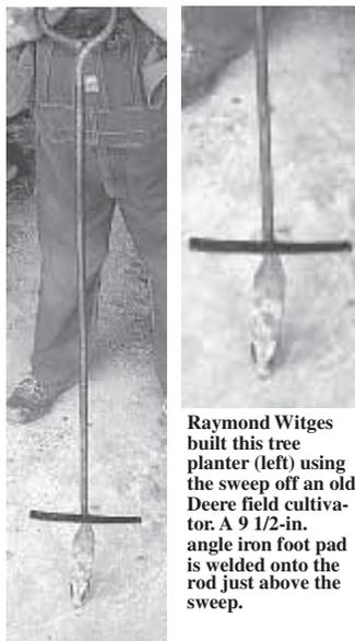
**Raymond Witges built this tree planter (left) using the sweep off an old Deere field cultivator. A 9 1/2-in. angle iron foot pad is welded onto the rod just above the sweep.**
