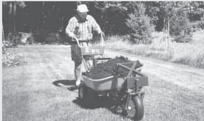
**Dump-style, sideways-mounted bucket can be bolted to wheelbarrow.**
