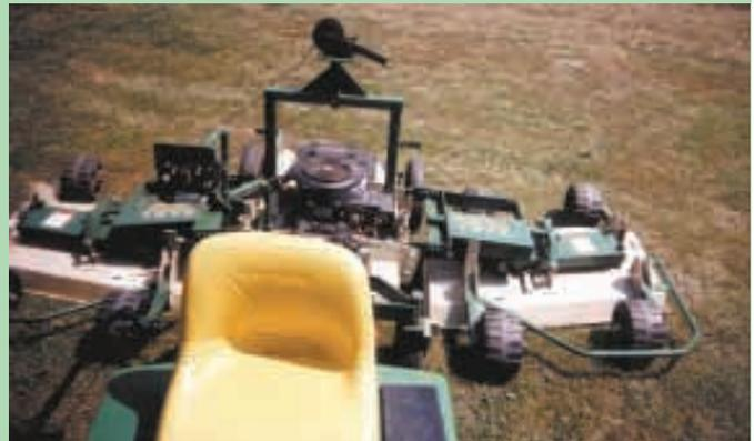
Middle deck is equipped with a Honda 16 hp engine that belt-drives wing decks.
