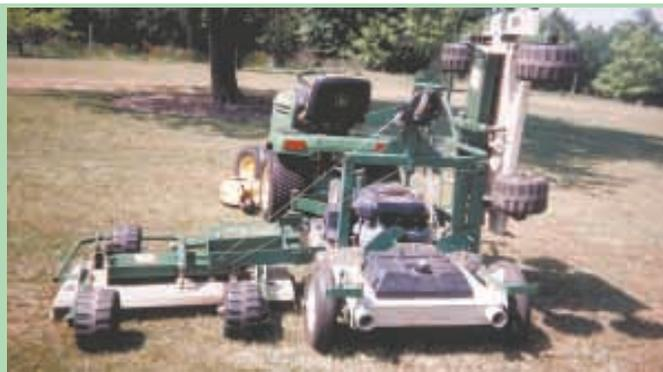
Pull-type mower is equipped with a “fake” middle deck that looks like a third mower but is actually the power source for two wing decks.
