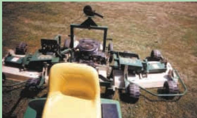
Middle deck is equipped with a Honda 16 hp engine that belt-drives wing decks.
