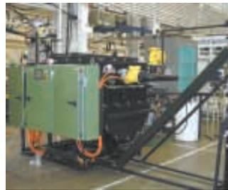
Prototype 1-ton system shown above can process 10 tons of tires, plastics or vinyl per hour into 17 million btu's of energy, with an 18:1 return on energy used in the process.
