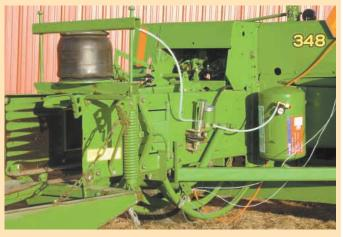
Airbaler kit replaces manual and hydraulic tensioning rods above bale chamber. Airbag mounts directly above bale chamber, fed by air from a small tank (at right in photo).
