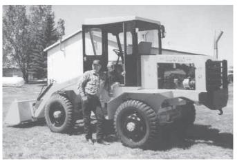
Mike Olson converted a surplus U.S. Army truck into this heavy duty front-end loader, flipping the axles so he could reverse the truck's direction.
