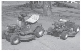
Bob Kessi uses his 42-in. cut MTD hydrostatic riding mower to pull a Craftsman 42-in. mower behind and off to one side. "It lets me make an 84-in. cut," he says.
