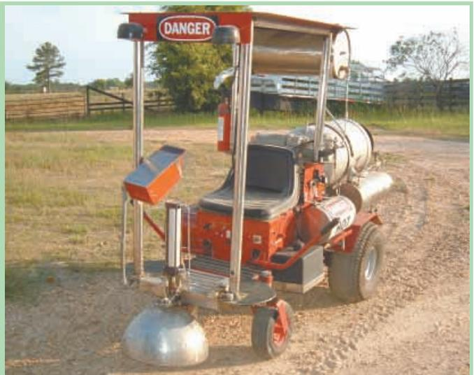
Machine injects 500-degree steam into center of fire ant nests at 40 to 50 lbs. of pressure. The steam kills the queen, which is all it takes to destroy a colony.
