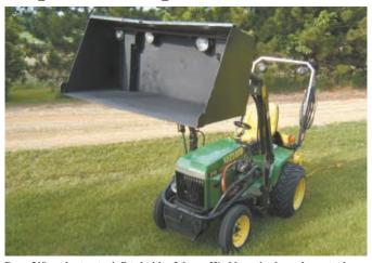
Deere 318 garden tractor is fitted with a Johnson Workhorse loader and an extra large, 1,000-lb. capacity bucket for snow and dirt. Note headlights at upper part of bucket.
