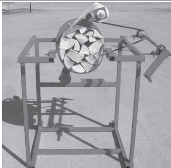
**New firewood bundler is easy to use. Wood is loaded into a hopper, then plastic is wrapped around it five or so times with a hand crank.**
