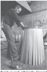
Barrels are made with lengths of tapered stave wood, bent and held together with steel hoops.
