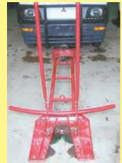
Tree Chopper was originally designed to be mounted to an ATV. Walnofer designed his own frame mount for his truck.
