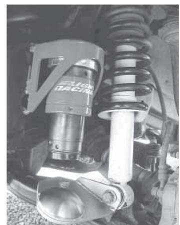
**Designed for full-size pickups, the JounceShock supplements a vehicle's existing shocks.**
