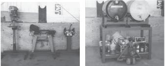
Hach bolted a wide metal stand onto most of his power tools (left). Oil storage rack consists of a storage table and a pair of metal "pallets" that each hold a 55-gal. barrel.
