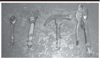
To use shop tools with his prosthetic arm, Matt Biel cut the handles off the tools and then welded a bolt onto each one. Then he threaded special adapters onto the bolts.
