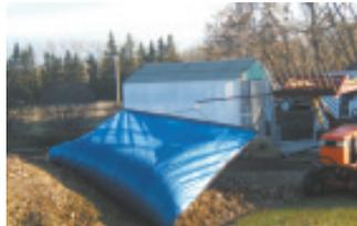
To unload leaves, he raises the loader up high and puts the tractor in reverse. As he starts to back up, tarp slides out from under the pile of leaves.
