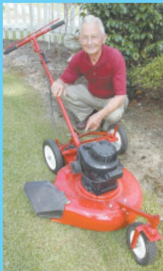
Furney Eubanks shows off the steering system he developed for push mowers. As the handle swivels, the deck slides left or right, so he can get close to obstacles without having to tilt or lift the mower.
