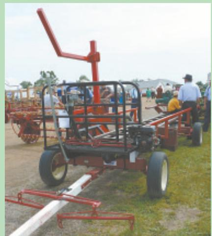
Self-powered bale carrier is designed for use with horses but can also be used behind pickups or tractors without hydraulics.
