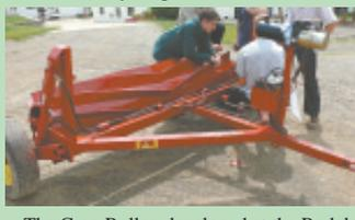
The Crop Roller, developed at the Rodale Institute and now being built by I&J Mfg., lays down and chops up crop residue, cover crops, or old hay crops prior to no-till or zone-till planting. The mat of residue it leaves on the ground holds down weeds. Units start at \$2,800.
