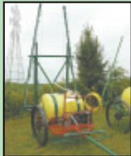
Boomtown also demonstrated this 110-gal. Hi-Rise Sprayer for produce, field crops and orchards. Equipped with a Honda motor, it produces 9.5 gpm and up to 580 psi with 24-ft. booms for up to 57 ft. of coverage. Booms can be raised to a 6-ft. height to spray corn. It's priced at \$1,982.
