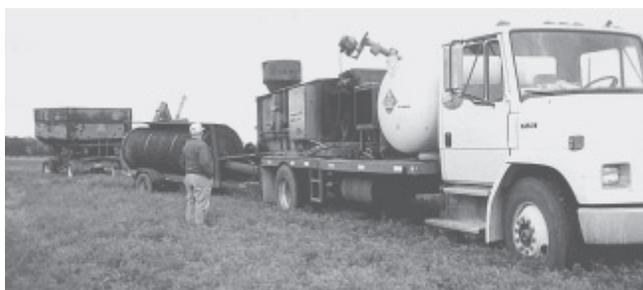
Grain roaster is heated by propane stored in tank on front of truck bed.
