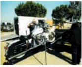
One-man motorcycle loader attaches to bed of pickup and can also be mounted on a trailer. It consists of a frame with an electrical-powered mounting rail in it.
