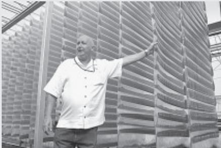
To produce hundreds of tons of algae, water is pumped through a series of clear plastic bags hanging from the roof of a greenhouse.
