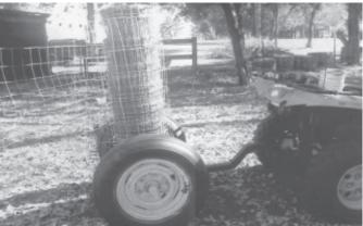
ATV-pulled, trailer-mounted fence unroller is built on the axle off an old boat trailer.
