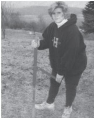
As operator lifts up on lever, it pinches into stake and pulls it out of ground.
