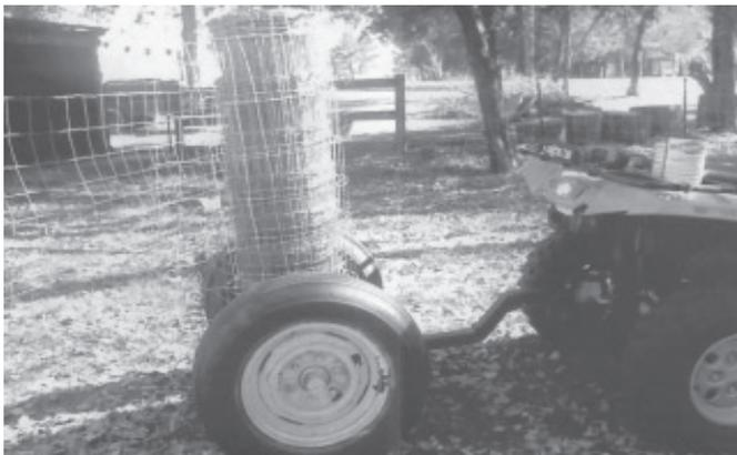
ATV-pulled, trailer-mounted fence unroller is built on the axle off an old boat trailer.
