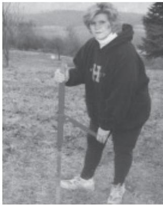
As operator lifts up on lever, it pinches into stake and pulls it out of ground.
