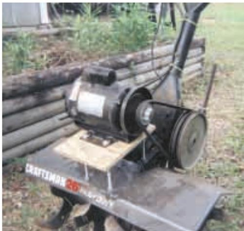
David Hunt bolted a 1/2 hp electric motor in place of the engine on his Sears rototiller. Pulley on motor belt-drives rototiller gearbox.
