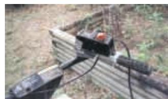
He ran motor's electrical cord to a switch that he mounted on the handle.
