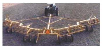
Harold Gleason tore apart four 9-ft. 6-in. New Holland Rolabar rakes to make this 4-ft. bar rake. It folds down to just 13 ft. 6 in. for transport.
