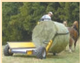
Operator uses hydraulics to lower bale arm to ground, then raises bale onto platform.
