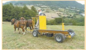
Horse-powered bale mover uses a mechanical braking system, but ground-powered hydraulics to pick up and handle bales.
