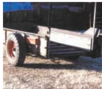
He pulled the beater off and bolted an angle iron frame to the beater mount holes.
