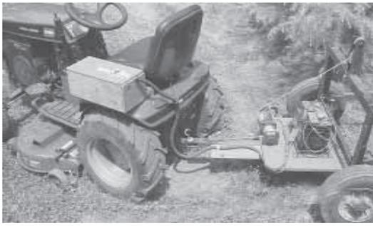
**Battery-powered electric winch provides lift on the 3-pt. hitch chassis.**
