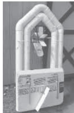
**Six direct-driven paddles are located in front, between the pedals (left). A 2-ft. sq. piece of high density styrofoam helps provide flotation.**
