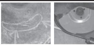
Steel patch reinforces the area where mower collects moisture from grass and starts to rust out or crack. It's a low cost alternative to replacing the entire deck.
