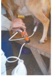
Main component of Grimmett's mini goat milker is a hand-operated fuel transfer pump.
