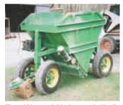
Honnold invented this rig to evenly distribute gravel along the trails of a shooting range. The variable speed electric motor slowly rolls gravel out in a 4-ft. wide path.
