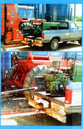
'Lets me use my pickup in place of a 50 to 60 hp. tractor," says Allan Cihar, Mosinee, Wis., who powers towed equipment behind his Ford F-250 with a stripped-down 1950's Deere 40 tractor that mounts in the box.
