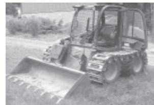
He also uses big buckets and a set of steel tracks on his JCB.
