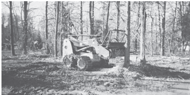
Art Bargabos uses a mulching head on his JCB skid steer loader to clear land.
