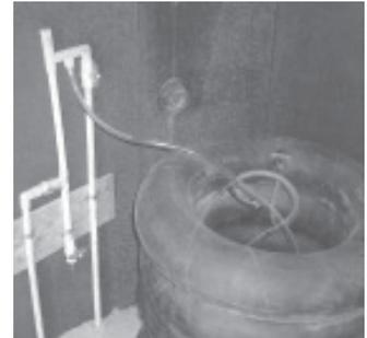
System consists of eight 55-gal. barrels that act as digesters. As it's generated, gas flows through two simple pvc manifolds that "scrub" it, draining moisture. Gas is stored in a stack of inner tubes.
