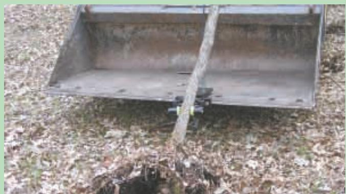
"Grabber" pulls brush by the roots. Several models are available, including one that clamps to the front edge of a loader bucket (above). A hand-powered version for post pulling and smaller brush is also available.
