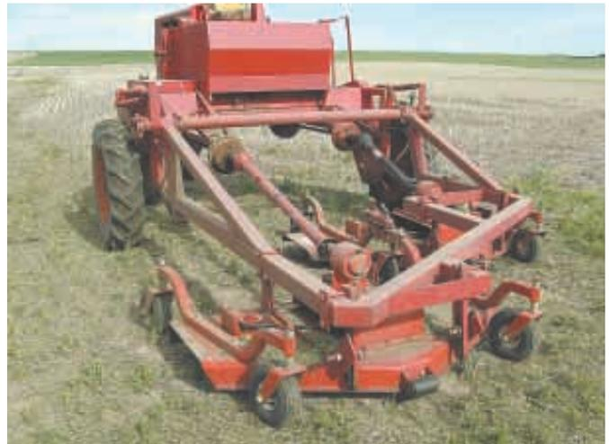
Swather is fitted with two 60-in., 3-pt. mounted finish mowers.
