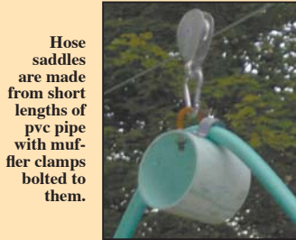
Darwin Keiper’s “hose trolley” lets him water any part of his garden with a 100-ft. long hose that never touches the ground.
