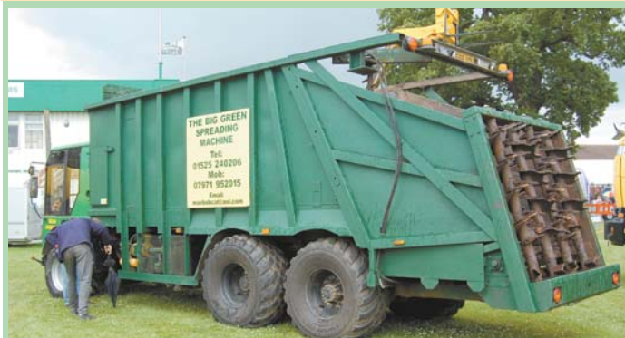
Four vertical spreader beaters mount on back of garbage truck. Truck’s original hydraulic-operated ram pushes manure onto chain-driven slat floor in front of beaters.
