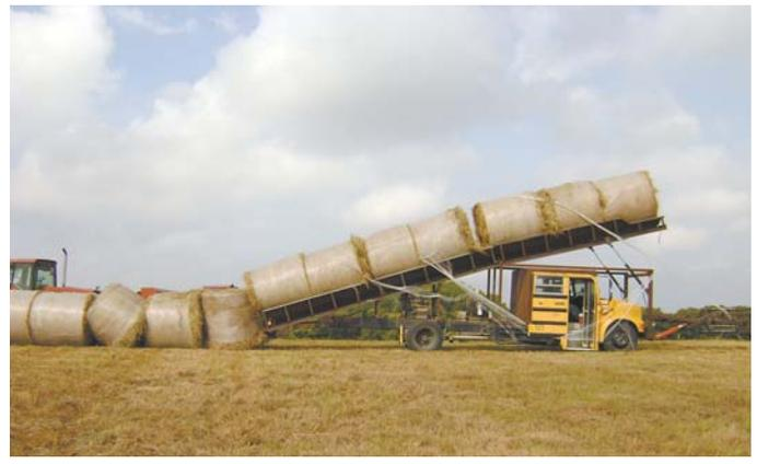
A separate 28 hp Kubota engine provides hydraulic power to clamp, lift and move bales up over top of cab and onto rear bale frame.
