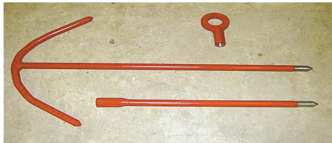
"Plug puller" consists of 5/8-in. cold-rolled rod, bent to an "anchor" shape. After pointed end is poked through plugup, extension and eye bolt are screwed on.
