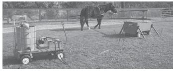
Traveling in a circle, horse drives a gearbox that powers a 600 rpm hydraulic pump which connects to the the ice cream maker.
