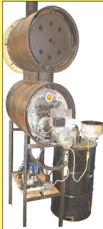
Tom Leue says his "Yellow Heat" burner efficiently burns used vegetable oil without clogging.
