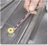
WrenchStops use removable magnetic inserts to reach bolts and nuts in hard-toreach places.
