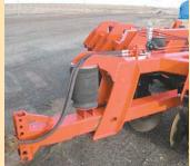
Air bags help disk float over on rough terrain of equal pressure..
