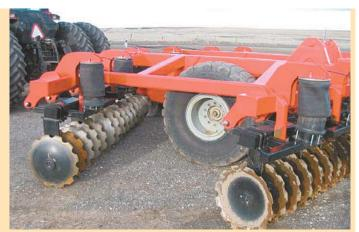
Disk's large truck tires provide extra flotation and minimize tire tracks.
