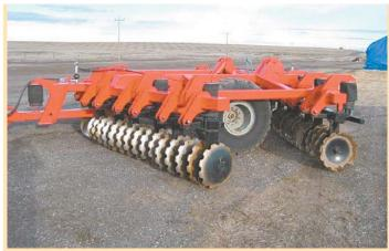
Heavy-duty "Rockzilla" disk uses truck air bags for suspension and to control gang
