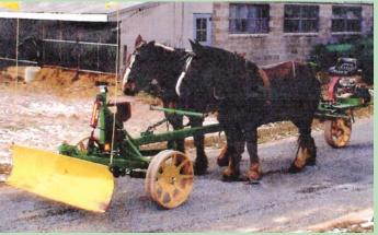
Lapp built this horse-powered snowplow from scratch. It has four hydraulic cylinders that are powered by an 8 hp motor on back.
