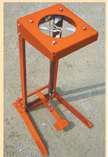
Bunching asparagus spears and other veggies is made easy with this semi-automatic buncher. It offers hands-free stretching and release of rubber bands.
