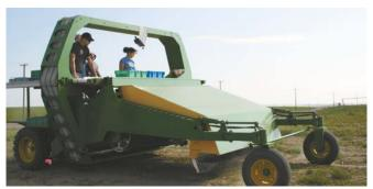
Asparagus harvester measures about 16 ft. long and 12 ft. wide. Workers stand ahead of the operator, selecting out asparagus spears as the conveyor drops them on the work table.
