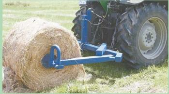
Unit can also be used to pick up and transfer bales.
