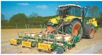
Developed in Ireland, the Samco planting system applies herbicide and plants the corn under 55-in. swaths of specially designed, degradable plastic.
