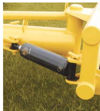
Blades are equipped with full hydraulic angle and offset control with double cylinders for on-the-go control.
