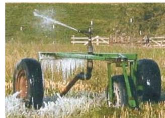
Pete Haugland uses his ATV to pull this home-built irrigation gun, along with 250 ft. of hose. There's no need to shut down or drain the system between mows.
