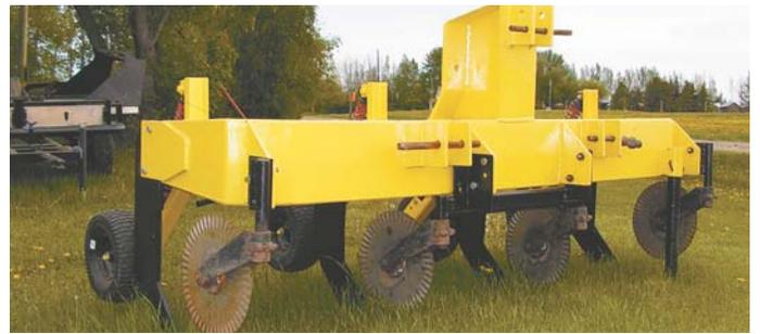
A 16-in. coultter precuts sod layers, and is followed by a shank and coil spring-mounted packer wheel.
