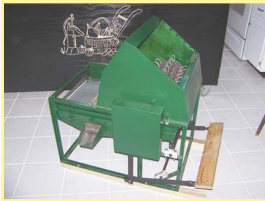
Small-scale thresher consists of a foot treadle, an enclosed threshing reel, and a winnowing screen.
