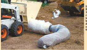
Instee Levee Builder lays an 18-in. high barrier 400 ft. long in less than an hour. An auger delivers material out the side to a 6-mil poly sock.
