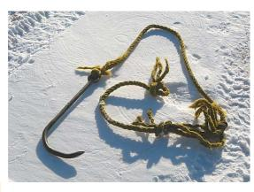
Designed to unplug round balers, hay hook is made from sucker rod bent into the shape of a giant fish hook.
