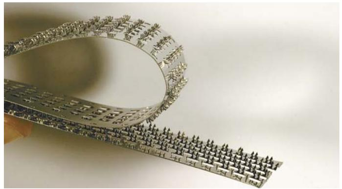
Steel "Velcro" consists of hooks and loops just like conventional Velcro, but is strong enough to hold machinery or building materials together.
