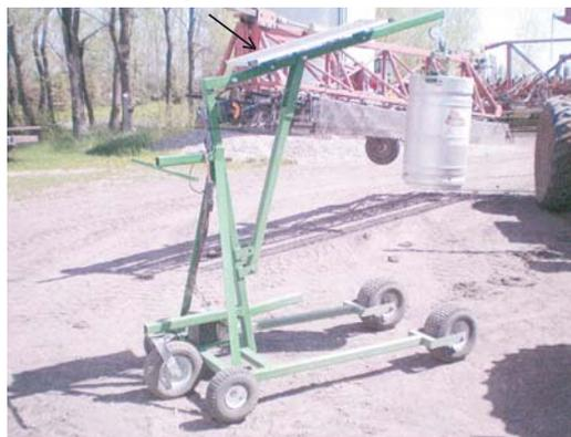
Mounted on top of hoist's boom, solar panel charges a car battery that powers a 12-volt electric winch. Arrow points to solar panel.
