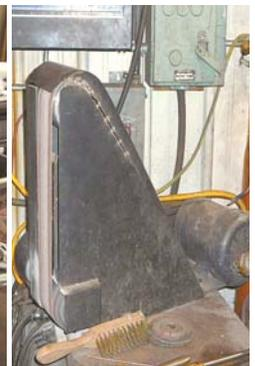
These big 3-phase shop tools are powered on single phase power by a VFD drive.
