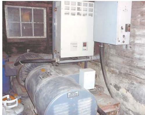
Myers coupled a 125 hp variable frequency drive to a 50 kw, 3-phase generator to power his shop.
