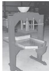
Shephard combined steel, plywood and a hydraulic pump to make a cider press.
