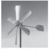
Stainless steel and aluminum frames give Miller's windmill stability and long life. tor heads from a windmill manufacturer and buys his towers locally.
