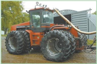
Flexible steel pipe runs from tractor exhaust back to cooler mounted on air seeder.
