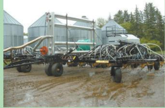
Exhaust coming off tractor at high temperatures must be cooled down to around 150 degrees before it's pumped into the ground.
