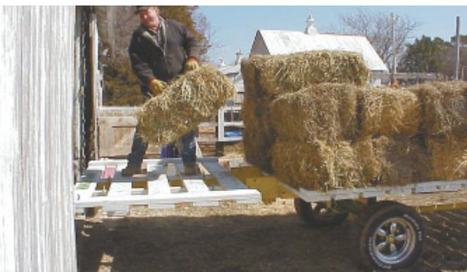
Wagon's back rack folds down for easy unloading of bales.
