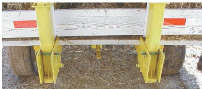
Hundertmark used parts from an old bean bar to build rack's hinge system.
